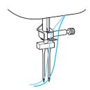
• The needle threader cannot be used with the twin needle. If the needle threader is used with the twin needle, the sewing machine may be damaged.
